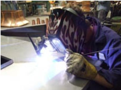
Showcasing C & R's abilities to work with a diverse group of materials, Dennis Jump works to weld together pieces of stainless steel.
